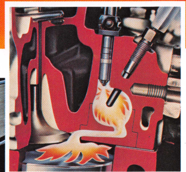
Electric glow plugs help provide efficient cold starting for the V8 diesel engine
